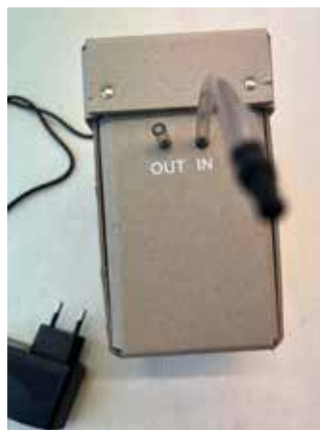
AIR-IN connect to vacuum frame AIR- OUT must not be blocked
