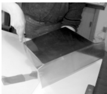
cut of excess film with a hobby knife
